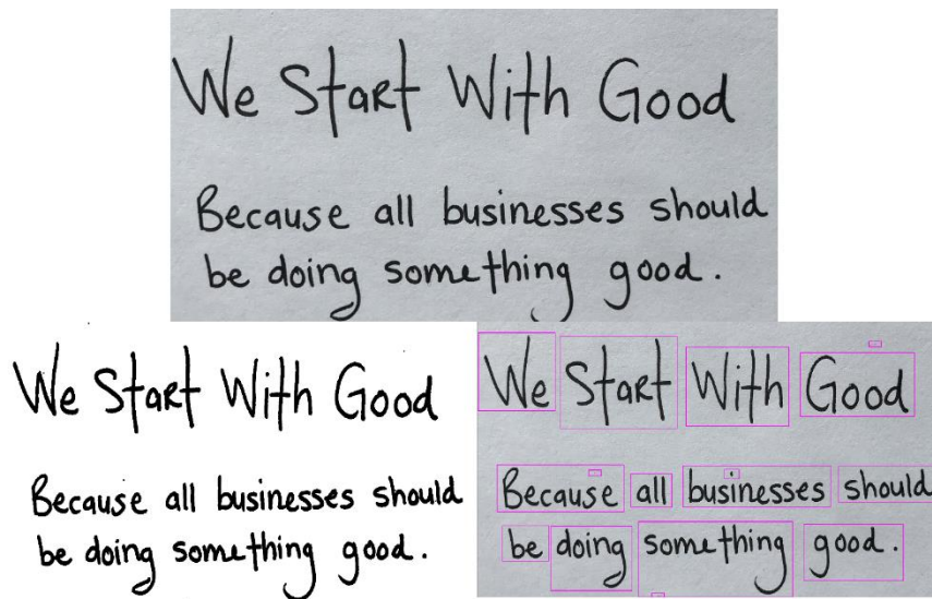
Figure 3 (a.) The image on the top is the original image (b.) image on the bottom left is the output of the image preprocessor (c.) image on the bottom right is the output of the word cropper
